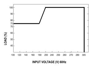
$\frak{M}$  De-rating is needed under low input voltage.
