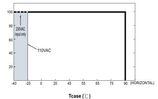
O If ELG-240 operates in Constant Current mode with the rated current, the maximum workable Ta is  $60^{\circ}$ C.
